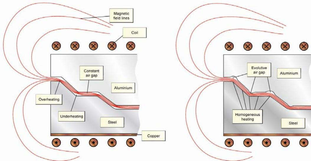
Fig. 5 Effect of air-gap on the magnetic field.
